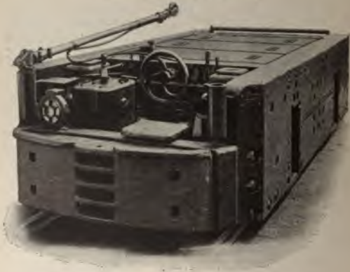
20-Ton, with Motors Centrally Hung
